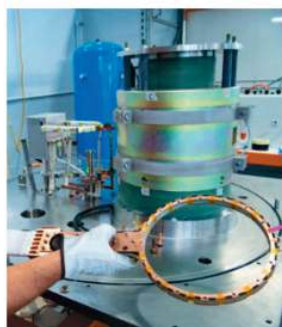
Figure 7. Scheme of HTS electric motor by the US company RTX
